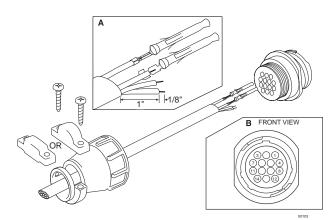
Figure 1. Connector Assembly
